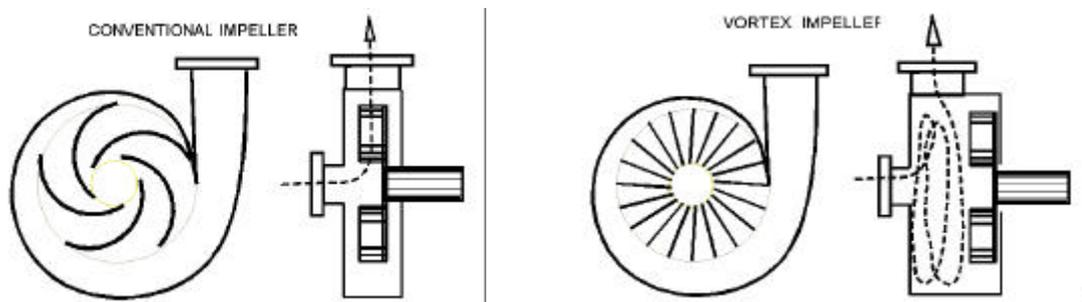
The advantage of this concept means that there is little, if any, direct physical contact between the particles and the rotating impeller thus allowing soft fragile particles to be transferred with significantly reduced attrition.
