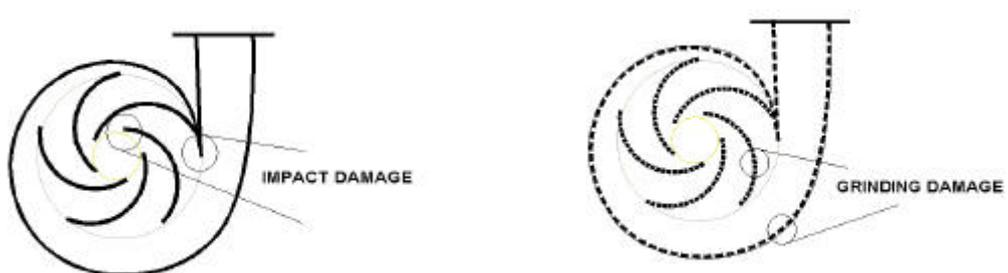
In impacts, the particles strike the surface at a very high angle and most of its kinetic energy is dissipated in fracturing the material surface, as well as itself. The damage intensity for brittle solids is related to the rotation of the impeller/particle hardness. If the particles are soft or fragile but with low hardness then particle damage may well be extensive.
