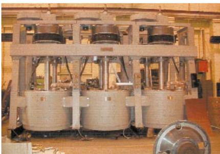
Picture 4. Broadbent expanded its portfolio with the refurbishment of six 25-year-old centrifuges for Snow White Sugar in Puerto Rico.
