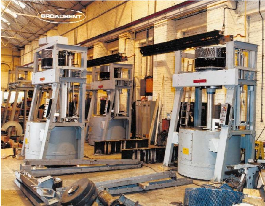
Picture 2. Refurbishment of a bank of centrifuges.
