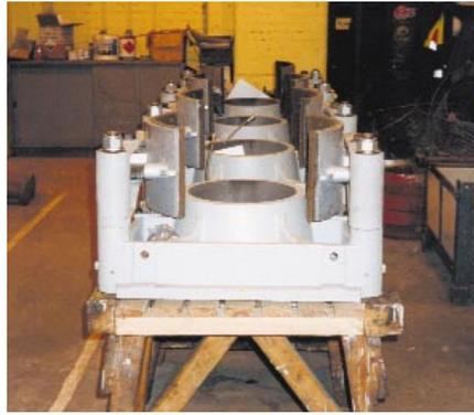
Picture 5b. The same machines at a later stage of reconditioning where the machines were dismantled into component parts.
