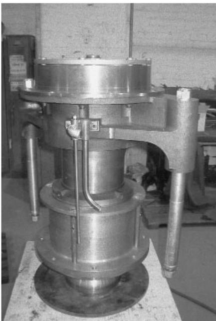
Picture 7c. Pictures 7a, b and c show a competitor's sugar discharge and head assembly being refurbished by BCSL.
