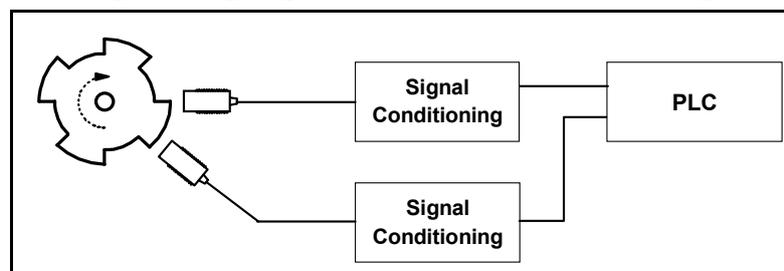
The scheme outlined in Fig 1 potentially has several defects. Firstly the PLC is the main control element which 'decides' if a fault exists by comparing the two speed signals and takes the necessary remedial action as defined by its program. However, there is only a single PLC and no checks are made on the correct operation of this PLC, so any failure or program error within the PLC may compromise safety.
