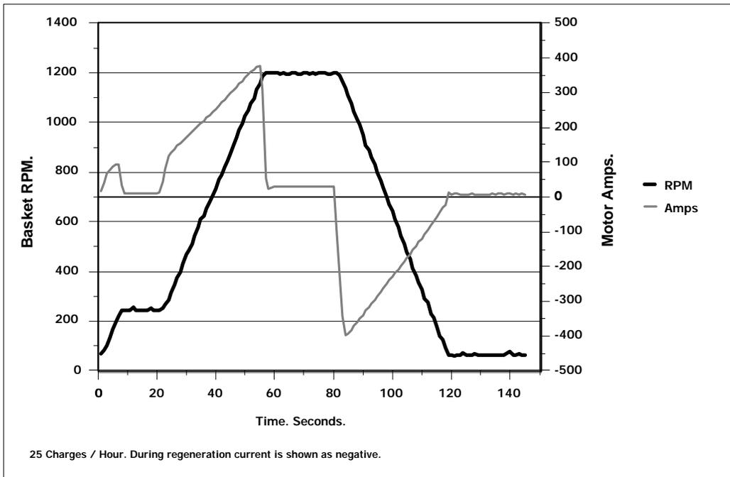
**Fig 6. Speed and motor current against time for an inverter drive.**
