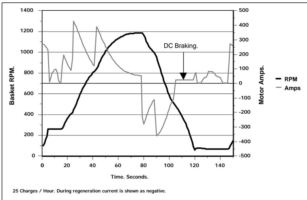
**Fig 5. Speed and inverter input current against time for an inverter drive.**
