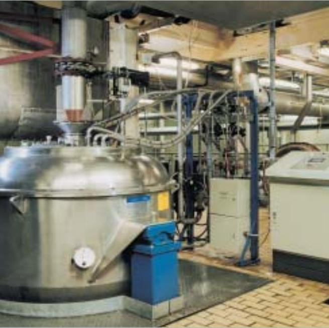
The **BROADBENT HIGH GRADE CONTINUOUS CENTRIFUGAL** uses processing techniques evolved from innovative technology developed by NQEA and their partners in the Australian sugar industry. These are combined with the proven design features of BROADBENT's low and intermediate grade continuous centrifugals to give batch results with continuous operation.
