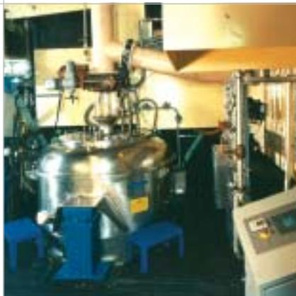
*Broadbent High Grade Continuous Centrifugals are ideally suited to replace batch centrifugals in low colour reduction applications, e.g. raw, affination & refined sugars*
